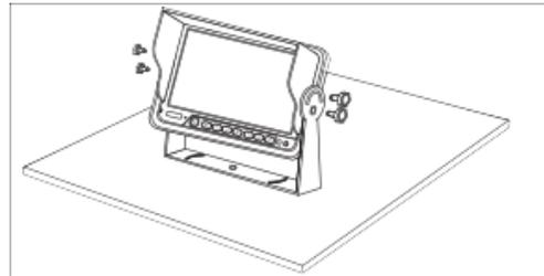
2. Finished the installation. Adjust the angle forward 30° to backward 30°. User can adjust a suitable angle by oneself.
